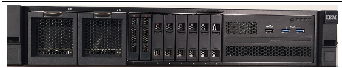
Figure 13 V9000 AC3 controller front view
