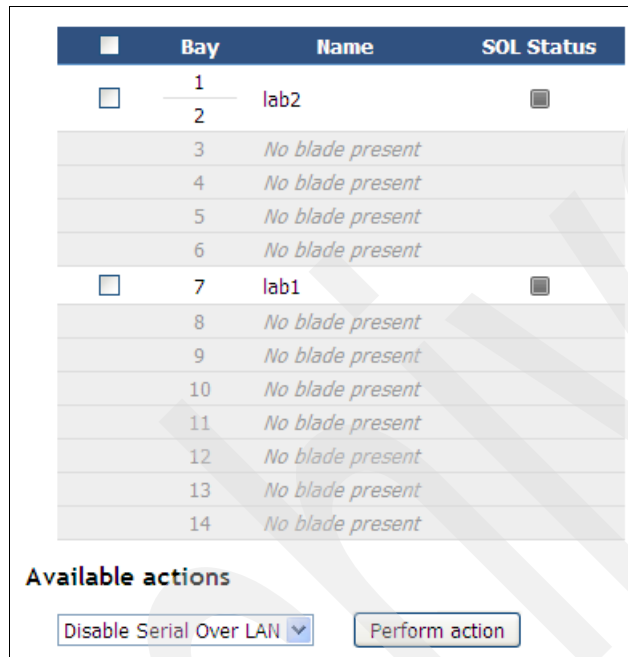
Figure 5-32 SOL disabled from AMM
