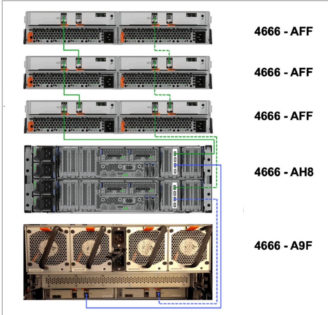
Figure 1-45 IBM FlashSystem 9500 system that is connected to expansion enclosure
