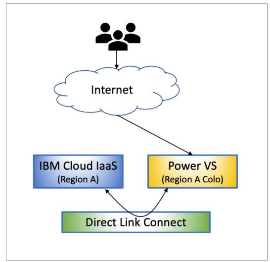
Figure 3-3 On-premises to Power Virtual Server directly
