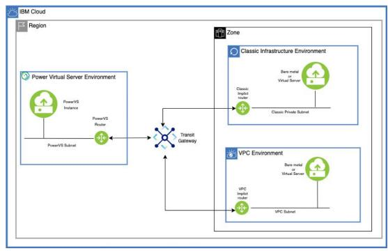
Figure 3-11 Power Virtual Server Cloud Connection with Transit Gateway
