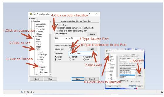
Figure 4-5 Set the source ports on PuTTY
