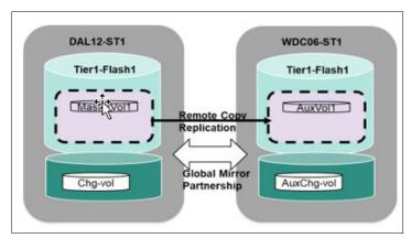
Figure A-4 Volume diagram, remote consistency group
