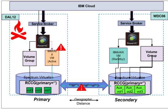
Figure A-23 Failover and failback diagram
