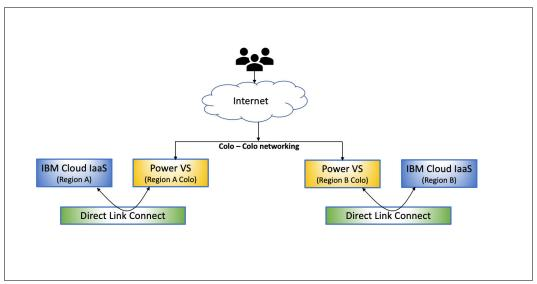
Figure 3-4 On-premises to Power Virtual Server (multiple COLOs)
