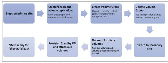
Figure A-7 DR recovery workflow diagram
