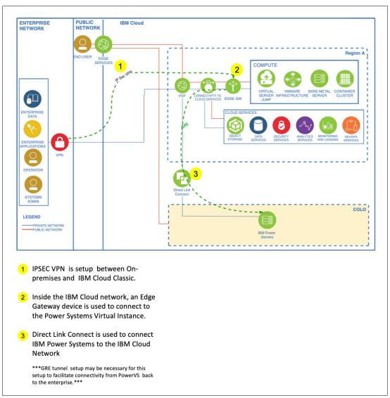
Figure 3-6 Private Connection using IPsec Virtual Private Networking, Direct Link, and Edge Gateway
