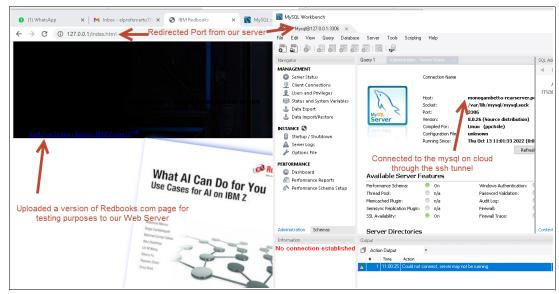
Figure 4-7 SSH tunneling access to apps
