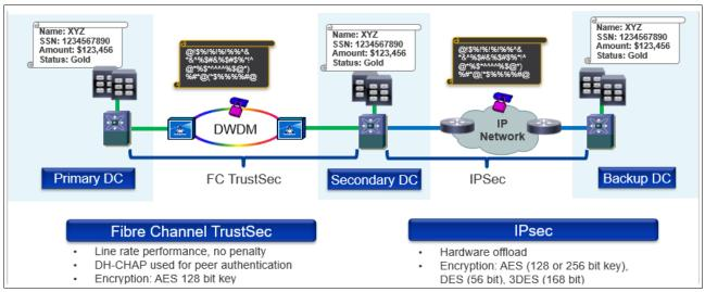
Figure 3-9 FC link encryption and IPsec features
