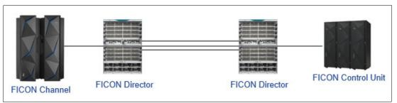
Figure 5-54 ISLs in a cascaded FICON topology
