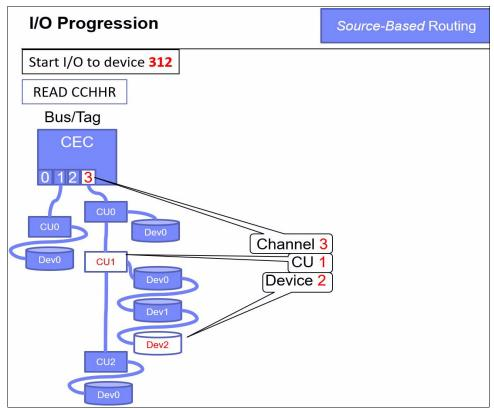
Figure 5-3 I/O in S/360: How a program controls the complete path for an I/O operation
