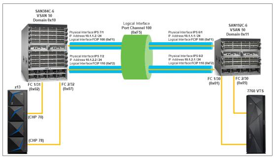
Figure 4-7 Cascaded VTS FCIP configuration with two physical interfaces
