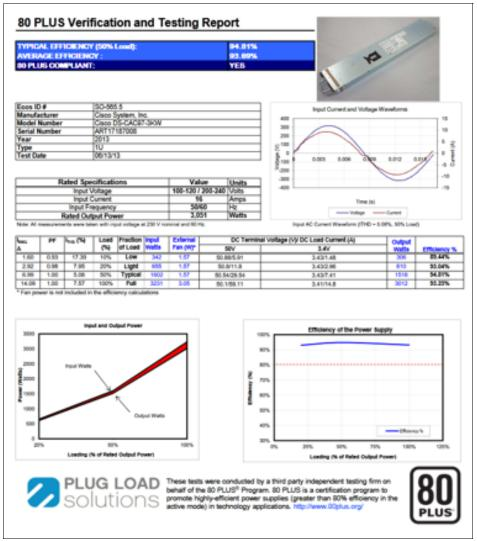
Figure 5-61 shows the official certification from the 80Plus organization for the IBM c-type 3 KW AC power supplies for a mission-critical director.
