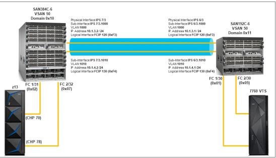
Figure 4-8 Cascaded VTS FCIP configuration with one physical interface and two subinterfaces
