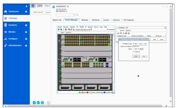
Figure 6-14 Configuring the IP address, Mode, and Preferred
