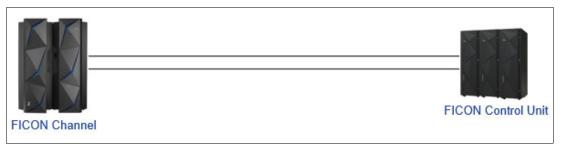
*Figure 5-48 Simple point-to-point topology*
