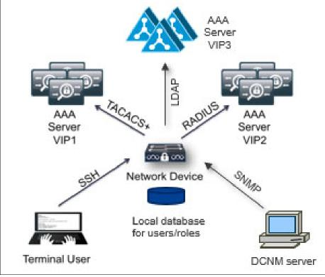
Figure 3-4 represents the secure access protocols and the options for both local and remote centralized AAA services.
