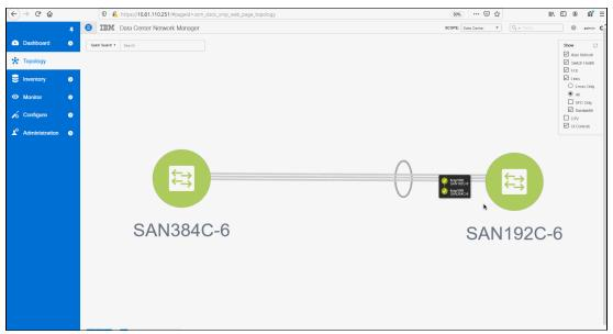
Figure 7-121 Showing the FCIP link
