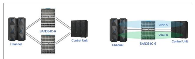
Figure 5-46 Physical versus logical redundancy
