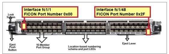
Figure 5-36 Interface numbering schema for a 48-port switching module in slot 1
