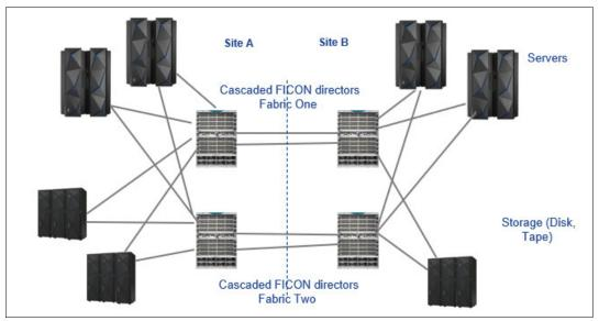
Figure 5-47 exemplifies a typical redundant deployment in a dual-site FICON environment.
