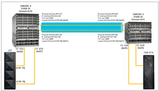
Figure 4-9 Cascaded VTS FCIP configuration with one physical interface and two FCIP interfaces with different TCP ports
