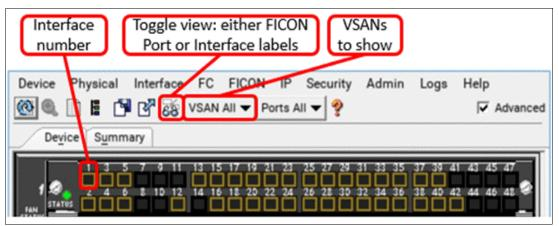
Figure 5-37 Default visualization from Device Manager with interface labels
