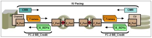
Figure 5-16 IU pacing flow control mechanism
