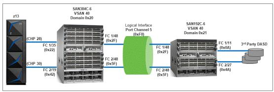
Figure 4-5 Cascaded FICON topology connection details
