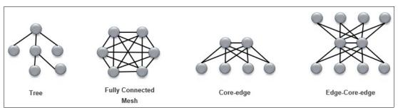
Figure 5-45 shows the most common FC network topologies.
