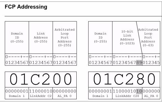
Figure 5-13 FCP link address and 10-bit addressing
