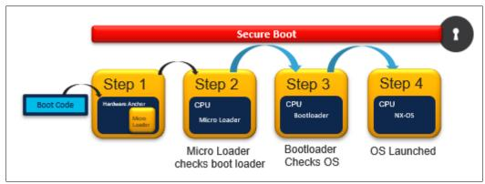
Figure 3-2 shows the secure boot process.
