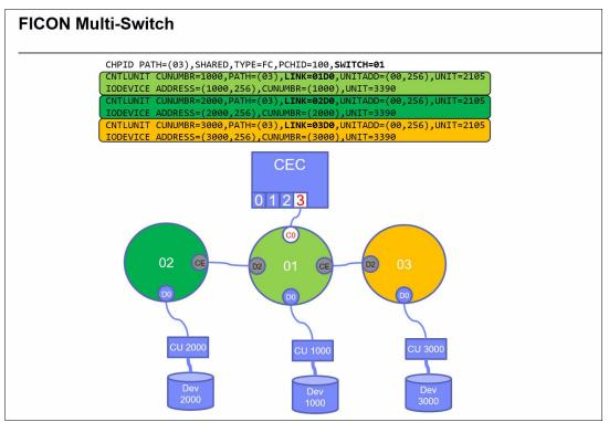
Figure 5-21 FICON multiple 2-switch paths from Switch 01
