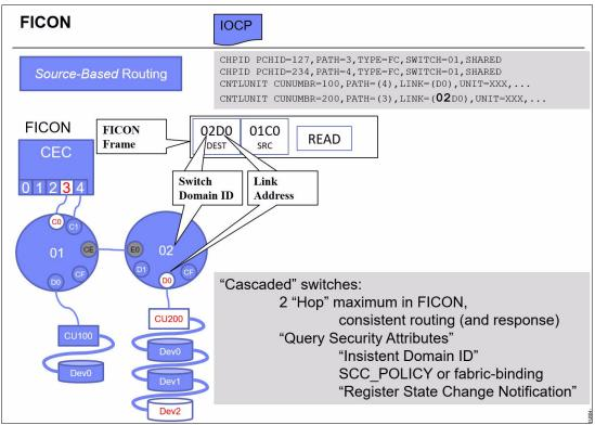
Figure 5-17 FICON I/O and the extended link address
