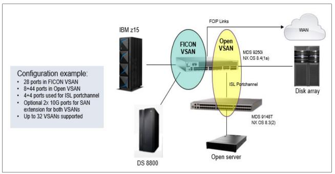
Figure 5-53 Port expansion in a FC/FICON intermix deployment scenario
