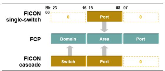
Figure 5-40 shows the static FCID allocation for switched and cascaded FICON topologies.
