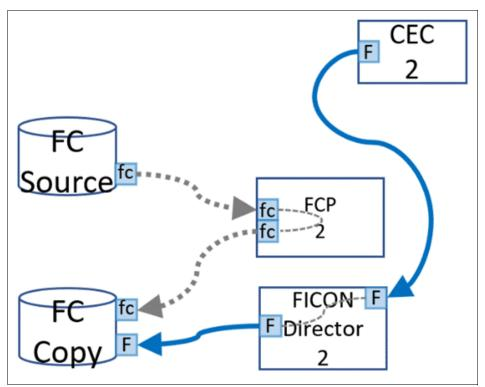
Figure 5-29 Storage replication: FlashCopy through an FCP SAN
