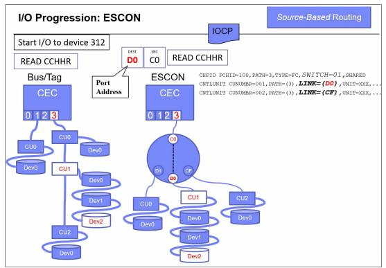
Figure 5-10 ESCON I/O and the SAN link address
