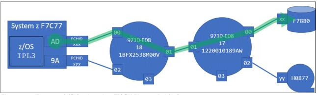
Figure 8-37 Diagram of I/O flow based on FICON Director Activity Report
