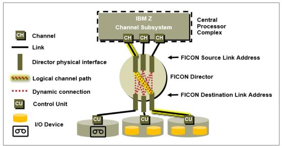
Figure 5-2 Logical channel path in a FICON switched fabric
