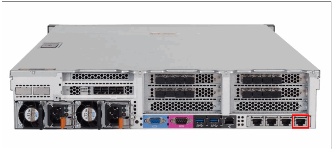
Figure 3-1 Location of the technician port on the SAN Volume Controller 2145-SV1 node
