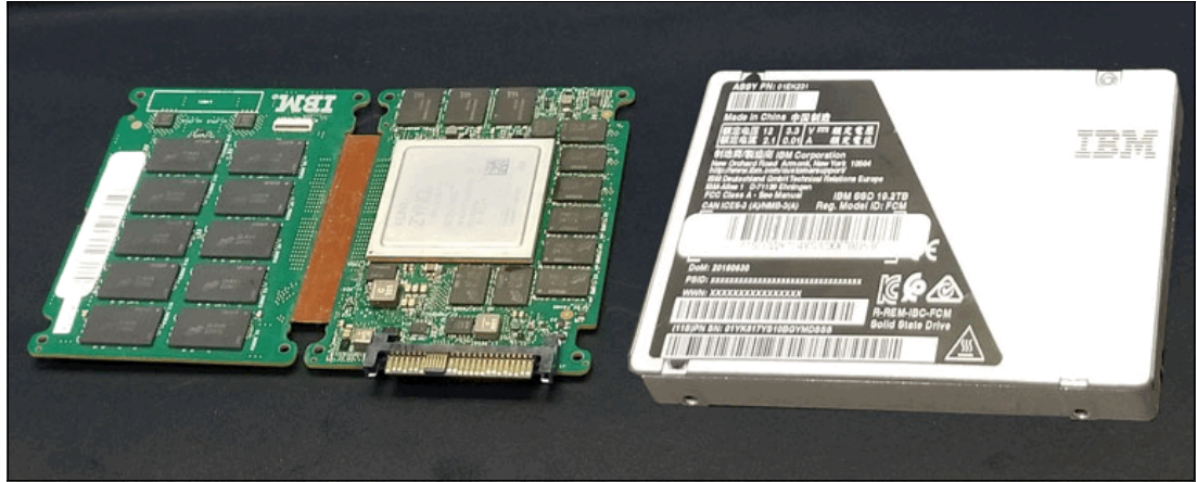
Figure 1-17 FlashCore Module (NVMe)
