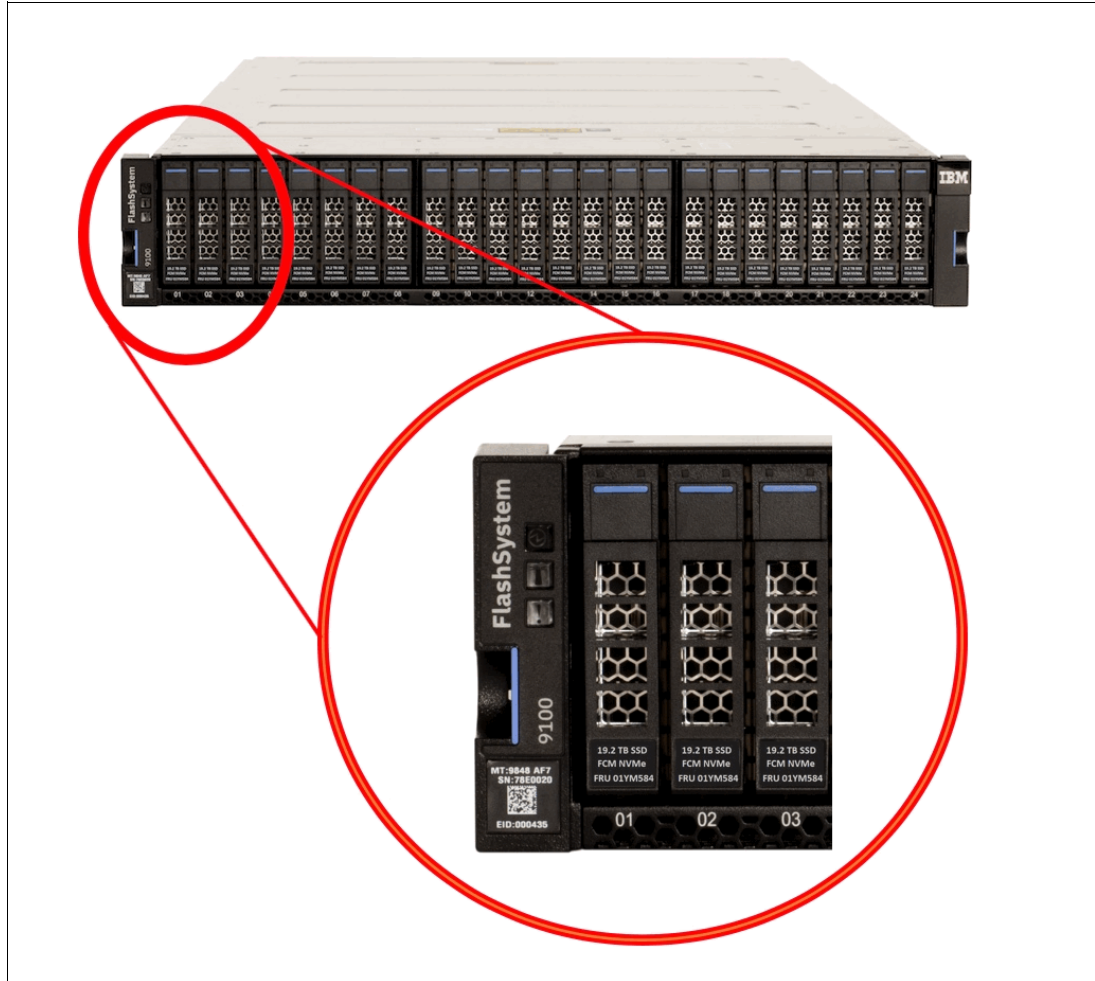
Figure 2 IBM FlashSystem 9100 bezel and FCM description.
