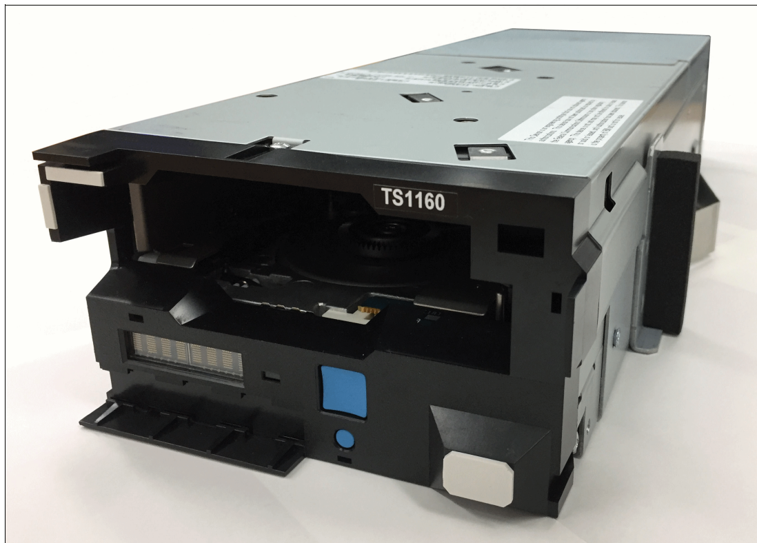
Figure 3-10 3592 60G tape drive
