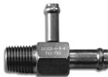
RA1K31-4-6-4 Fitting, T, 1/4" NPT, 3/8" hose, 1/4" hose T For instrument inlet and outlet ports with T for gauge. Replaces - Airborne PN. 1K31-4-6-4
