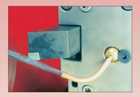
LolliPop nozzle shown installed in lathe turret.
