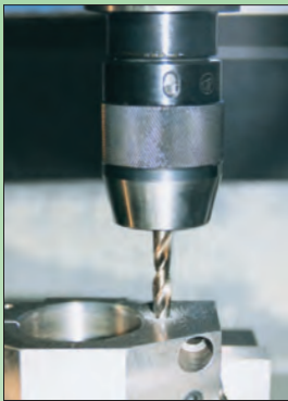
1 Drill coolant passage, leaving reaming allowance.
