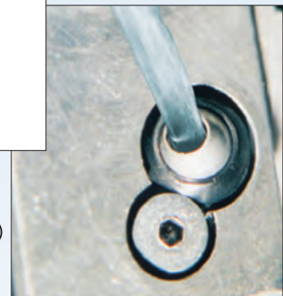
BlackEye installed on quick change turning tool.
