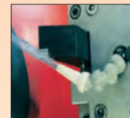
TYPE 2 OddBall attached to 1/4" Snap-Loc** hose.
