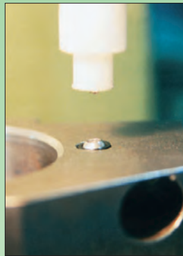
3 Press in JiffyJet until body is flush.
