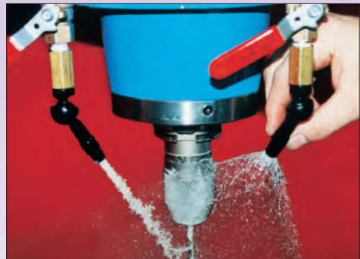
MillJets shown installed on Vertical Machining Center showing wide and narrow spray.
