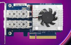
The dual-port 10GbE SFP+ high-speed expansion card can support a highperformance Remote Direct Memory Access (RDMA) protocol. It allows the data to bypass the network driver and communication layer directly through the application server's memory buffer and storage device, which greatly reduces the host CPU load. The NAS can handle more processes with such offload.
