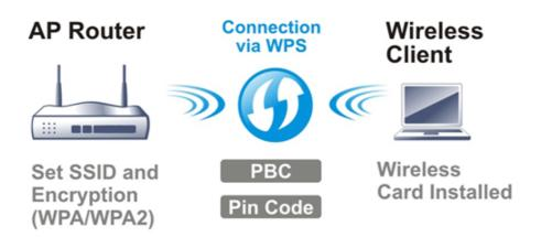
It is the simplest way to build connection between wireless network clients and VigorAP 918R. Users do not need to select any encryption mode and type any long encryption passphrase to setup a wireless client every time. He/she only needs to press a button on wireless client, and WPS will connect for client and VigorAP 918R automatically.
