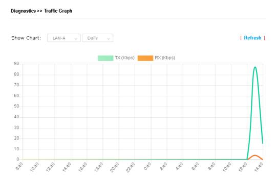
The horizontal axis represents time; the vertical axis represents the transmission rate (in kbps).
