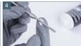
4 Grease paint needle around the needle packing area
