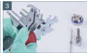
3 And finally, unscrew fluid tip with the ring spanner.
