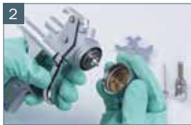
2 Then disassemble the air cap.
