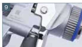
9 Grease visible part of air piston rod
