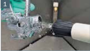
1 Insert spray gun body
