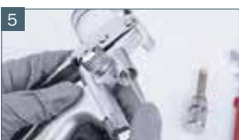
5 Insert paint needle
