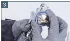
3 Assembly of the air cap. Air cap marking must be legible.
