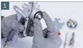
1 Assembly of the fluid tip
