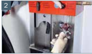
2 Blow dry spray gun and material passage
