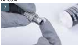
7 Grease thread of material flow control screw
