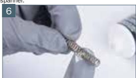
6 Grease and insert paint needle spring
