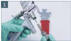
1 First remove paint needle.
