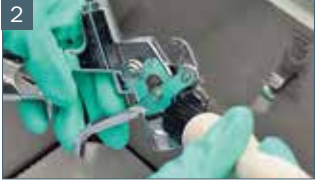
2 Connect air connection to air inlet
