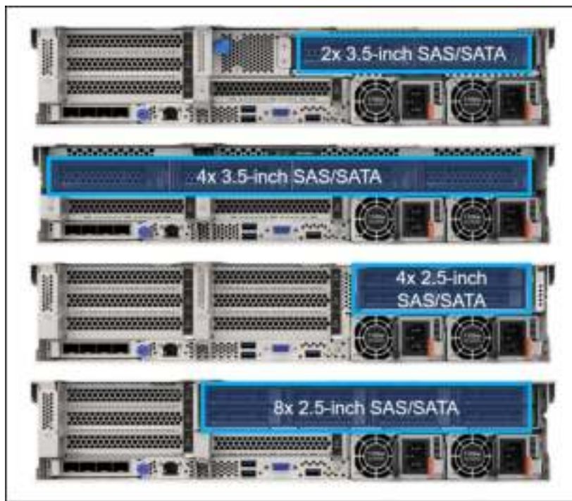
Figure 9. Rear 2.5-inch and 3.5-inch drive bay configurations
