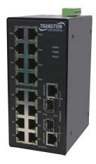
The SISTM1040-262D-LRT-B switch is a (16) port managed hardened switch with (2) copper ports or (2) dual speed SFP slots supporting Fast Ethernet to Gigabit Ethernet speeds. The (2) SFP slots provide the ultimate flexibility by allowing SFP fiber connections at different speeds and at a variety of communication distances. The ports can also be used in a redundant ring for maximum network reliability
