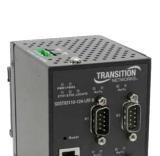
Transition Networks serial device server provides the ability to communicate serial data across an Ethernet network. The SDSTX3110-124-LRT-B contains (2) 10/100Base Fast Ethernet ports that can be configured to one or multiple redundant servers. Security of the data transmission is assured through HTTPS, SSH, and SSL data encryption.
