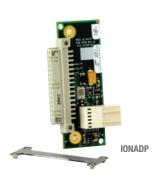
The IONADP is an adapter card that allows the ION Platform chassis to be backwards compatible with Point System<sup>™</sup> modules. This adapter is designed to sit between a Point System<sup>™</sup> module and the backplane of the ION chassis. The purpose of the IONADP is to lengthen the Point System<sup>™</sup> module so it can be securely mounted in an ION chassis while also connecting to the backplane allowing the ION chassis to power the Point System<sup>™</sup> module.
