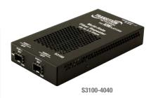
The ION S3100 is a stand-alone fiber to fiber media converter. It is protocol independent and supports data rates from 100Mbps to 2.5Gbps through two open SFP slots. This any-rate to same-rate converter can be used to perform reliable and cost-effective single mode to multimode fiber conversion or it can be used to provide wavelength conversion in CWDM applications.
