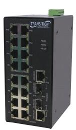
The SISTF1040-162D-LRT is a high port density switch suitable for use as an aggregation switch in a challenging environment. The two gigabit speed combo ports provide the ultimate flexibility by allowing copper or fiber SFP uplink ports. The two uplink ports can also be used in a redundant ring for maximum network reliability. The switch has redundant input power connections, and a fault alarm relay to ensure safe reliable operation in temperatures between -40°C and +75°C.
