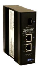
The SI-IES-121D-LRT is a (3) port unmanaged hardened PoE+ injector / converter that adds up to 30 Watts of power from its (2) PoE+ ports onto 2 network segments. The gigabit speed SFP slot provides the ultimate flexibility by allowing fiber SFP uplink ports with varying communication distances.
