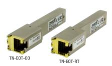
The TN-EOT-xx Series is an Ethernet Extender in a standard SFP form factor, it provides the ability to leverage the existing 2-Wire or Coax cable infrastructure to extend the Ethernet service. It can extend the Ethernet service on 2-wire with distances up to 400 meters at 200Mbps bi-directional data rate or extend Ethernet on Coax cabling with distances up to 500 meters at 300Mbps bi-directional data rate.
