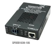
The SPOEB Series is a 10/100 Ethernet copper to fiber PoE media converter that enables enterprises to provide power to network devices over the existing CAT5 data connection.
