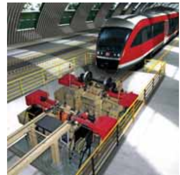
Hegenscheidt Underfloor Wheel Lathe
