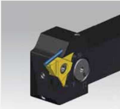
Coolant supply directed to the rake face
