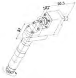
GSE-507-DE End Drill/Mill Collet Size: ER08, ER11 Output: 1:1 Double Ended
