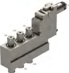
BSA-2010 Angled Drill/Mill Collet Size: ER16 Output: 1:1 Adjustable 0-21° Interferes with adjacent tooling position when used at angle A32 L32
