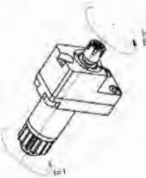
GSE-3307-L-3X End Drill/Mill Collet Size: ER08 Output: 1:3
