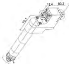
GSE-306-DE511 End Drill/Mill Collet Size: ER11 Output: 1:1 Double Ended L 4 25 L 4 32
