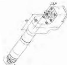
GSE-306-DE512 End Drill/Mill Collet Size: ER11 Output: 1:3 High Speed Double Ended L 4 25 L 4 32
