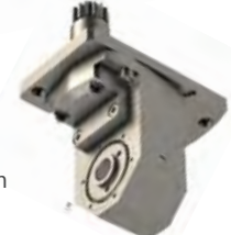
MSH-507 Gear Hobbing ID Size: Ø4.5mm Output: 1:1 Hobb OD: Ø12mm Hobb Thickness: 10mm
