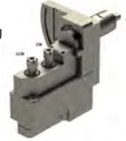
B07-GSA-207-2X Angled Drilling / Milling Arbor Size: ER11 Output: 1:2 Adjustable 90° High Speed Machine: B01/02/07
