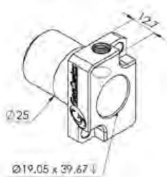
GSS-1530 Slitting Saw Arbor Size: ER11 Output: 5:3
