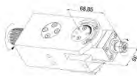
DE13-0042 Angled Drilling / Milling Collet Size: ER11 Output: 1:1 Adjustable 0-90°
