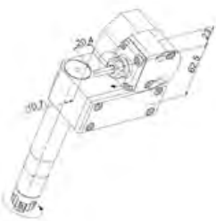
GSA-507 Angled Drill/Mill Collet Size: ER11 Output: 1:1 Adjustable 0-180°
