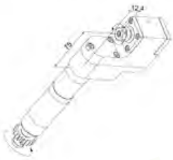
GSE-306-SE512 End Drill/Mill Collet Size: ER11 Output: 1:3 High Speed
