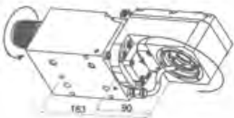
DE20-W15 Thread Whirling Ring: Utilis Output: 1:1 9 or 12 Insert Cutter, Flight Circle Ø12mm Coolant-Thru (Ext)
