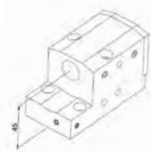
VDF-205-S-2 Tool Holder Tool Size: Ø19.05mm Coolant-Thru
