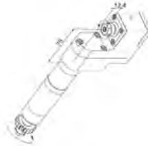
GSE-306-SE312 End Drill/Mill Collet Size: ER11 Output: 1:3 High Speed L 6 32
