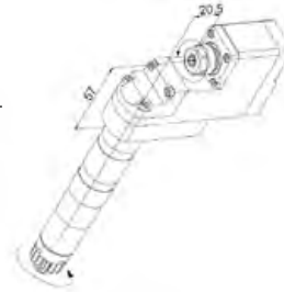
GSE-507-DS End Drill/Mill Collet Size: ER11 Output: 1:1 Double Ended
