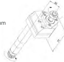
GSS-250-13 Slitting Saw Arbor Size: Ø13mm Output: 2:1
