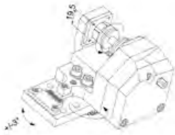
MSH-132-10 Gear Hobbing ID Size: \varnothing 10\text{mm} Output: 3:1 Adjustable \pm 3^\circ
