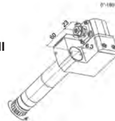
GSC1010-GS Cross Drill/Mill Collet Size: ER16 Output: 1:1 L 6 32
