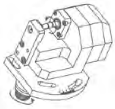
KSH-133-035 Gear Hobbing ID Size: Ø3.5mm Output: 1.588:1 Adjustable 0-30°
