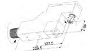
DE20-0011 Drilling / Milling Collet Size: ER16 Output: 1:1
