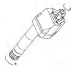
GSE-316-GS End Drill/Mill Collet Size: ER16 Output: 1:1
