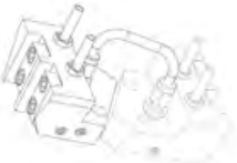
VTF1510-D Tool Holder Tool Size: 10x10mm Coolant-Thru Requires Y-Axis
