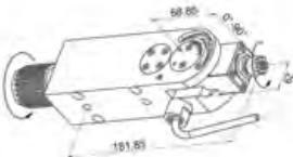
DE20-0004 Angled Drilling / Milling Collet Size: ER11 Output: 1:1 Coolant-Thru (Ext) Adjustable 0-90°
