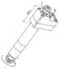
GSC-607-2X Cross Drill/Mill Collet Size: ER11 Output: 1:2 High Speed
