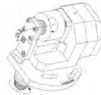
KSH-132-27-17 Gear Hobbing ID Size: Ø10mm Output: 1.588:1 Adjustable 0-20°
