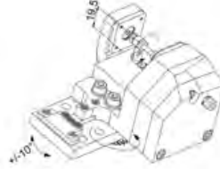
MSH-133-035 Gear Hobbing ID Size: \varnothing 3.5\text{mm} Output: 1:0.762 Adjustable \pm 10^\circ
