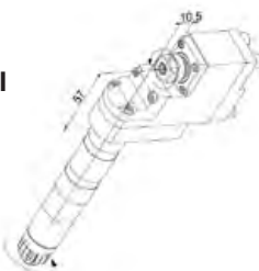
GSA-507 Angled Drill/Mill Collet Size: ER11 Output: 1:1 Adjustable 0-180°
