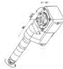
GSS-450 Slitting Saw Arbor Size: Ø16mm Output: 4:1
