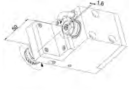
MSE-106-KM End Drill/Mill Collet Size: ER11 Output: 1:1 Coolant-Thru
