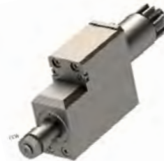
GSS-1530 Slitting Saw Collet Size: ER11 Output: 5:3 Max Tool Ø63mm Max Width 2mm
