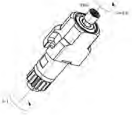
MSC-507-4X End Drill/Mill Collet Size: ER08 Output: 1:3.8 High Speed
