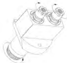
SV32-TSC-210 Cross Drill/Mill Collet Size: ER16 Output: 1:1
