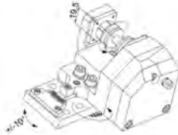
MSH-132-S-035 Gear Hobbing ID Size: \varnothing 3.5\text{mm} Output: 3:1 Adjustable \pm 10^\circ
