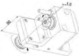
MSE-106-2X End Drill/Mill Collet Size: ER11 Output: 1:2 Coolant-Thru High Speed
