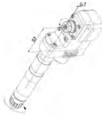
GSE-708 End Drill/Mill Collet Size: ER11 Output: 1.65:1
