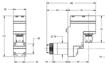
STA-R146-E16 End Drill/Mill Collet Size: ER16 Output: 1:1
