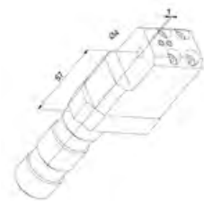
GDF-901-S1X4 Tool Holder Tool Size: Ø4mm
