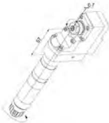
GSE-707 End Drill/Mill Collet Size: ER11 Output: 1:1
