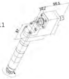
GSE-507-DS End Drill/Mill Collet Size: ER11 Output: 1:1 Double Ended
