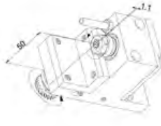
MSA-303 Angled Drill/Mill Collet Size: ER11 Output: 1:1 Adjustable 55-90°
