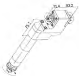
GSE-306-DE511 End Drill/Mill Collet Size: ER11 Output: 1:1 Double Ended
