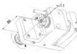
MSE-106-2X End Drill/Mill Collet Size: ER11 Output: 1:2 Coolant-Thru High Speed
