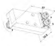
MSC-407 Cross Drill/Mill Collet Size: ER11 Output: 1:1 Requires Y-Axis
