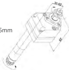
GSS-450 Slitting Saw Arbor Size: Ø16mm Output: 4:1
