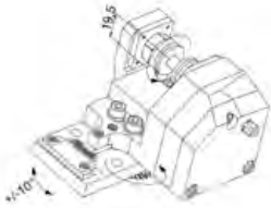
MSH-132-S-035 Gear Hobbing ID Size: \varnothing 3.5\text{mm} Output: 3:1 Adjustable \pm 10^\circ
