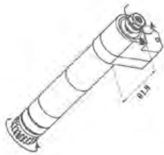
GSC-510-L-3X Cross Drill/Mill Collet Size: ER11 Output: 1:3 High Speed L 6 32
