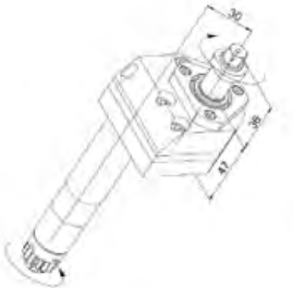
GSS-250-15 Slitting Saw Arbor Size: Ø15.875mm Output: 2:1
