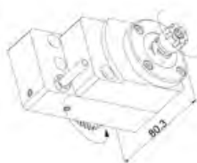
MSC-106-2X Cross Drill/Mill Collet Size: ER11 Output: 1:2 Coolant-Thru High Speed
