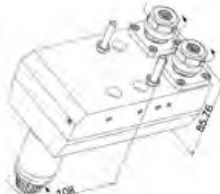
KSC-510-10 Cross Drill/Mill Collet Size: ER16 Output: 1:1.5 Coolant-Thru Y-Axis Required 10mm Offset
