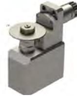
BSC-2330 Cross Drill/Mill Collet Size: ER11, ER16 Output: 1:1 Requires 2 Tool Positions A32 L32
