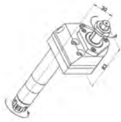
GSS-250 Slitting Saw Arbor Size: Ø16mm Output: 2:1
