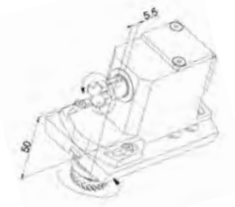
MSF-130 End Drilling/Milling Collet Size: Ø13 Output: 1:1 Adjustable ±20°
