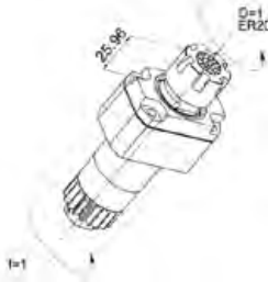
GSC-1113 Cross Drill/Mill Collet Size: ER20 Output: 1:1 A32 L32
