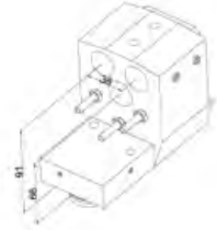
CDF-901-AR Tool Holder Tool Size: Ø25.4mm Coolant-Thru Y-Axis Required
