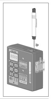
Stand the pump upright on a level surface and set the pump running. Set the pump flow rate to approximately 1.5 l/min. The built in flow indicator rotameter can be used to make this setting as only an approximate flow rate is required.
