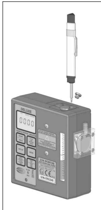
Stand the pump upright on a level surface and set the pump running. Set the pump flow rate to approximately 1.5 l/min. The built in flow indicator rotameter can be used to make this setting as only an approximate flow rate is required.
