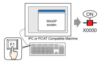
Press the function key on the keypad while WinGP is running to operate the switch feature. In the function settings, allocate a switch feature to a function key on the keypad. The function settings include [Global Function] where switch feature can be set as a function key common to project data or [Local Function] where different switch features can be set for a function key on each base screen.
