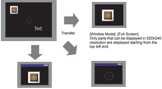
[Window Mode]: [Window Screen] [Specify Display Position] is specified, [X Coordinate] is 0, and [Y Coordinate] is 0 Only parts that can be displayed in 320X240 resolution are displayed starting from the top left end.
