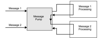
If it takes a long time to process Message 1 at this point, the message pump does not return and the message pump processing 2 cannot be performed.
