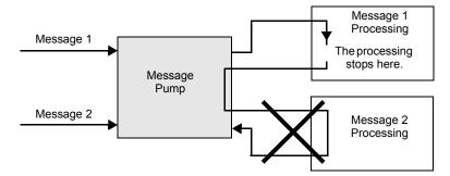
In such case, force the operation of the message pump. (Referred to DoEvents in VB and GetMessage() and DispatchMessage() in , VC)
