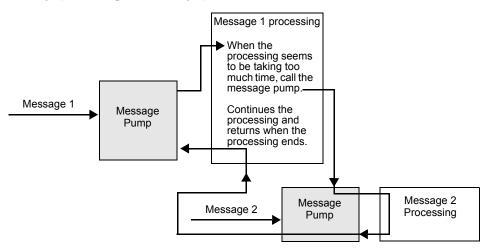
Windows applications are designed based on applications to operate the message pump properly. In order to prevent such an event as shown in the example, WinGP SDK operates the message pump in the function when processing takes too long.
