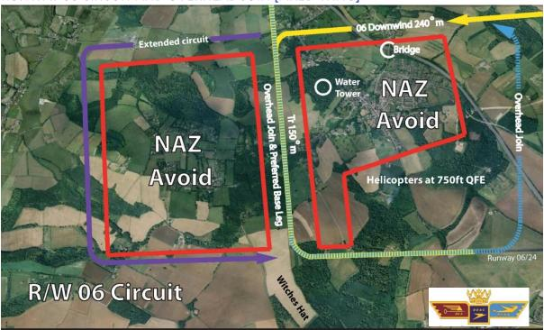
Circuit Height 1000ft QFE. Fly downwind leg between Motorway Bridges. When abeam Water Tower turn Base Leg aiming for 'Witches Hat'.
