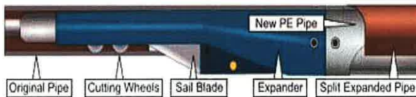
Figure A5-5 Pipe Splitting Equipment
