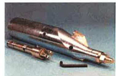
Figure A5-4 Pipe Splitting Bursting Head
