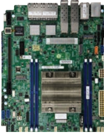
Intel® Xeon® D SoC, 4/14/16-Core, Quad 10GbE LAN Intel® Quick Assist Technology
