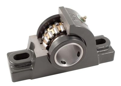
The PPI Type E pillow block bearing was designed specifically for the challenges of multiple conveyor applications. That's why our Type E bearing utilizes a double row spherical bearing that makes a misalignment of  $\pm$  2 degrees possible. This allows the bearing to be more forgiving of mounting positions that are less than perfect. Additionally, a double lip nitrile contact seal provides the necessary protection from the heavily contaminated applications, common to the conveyor industry.
