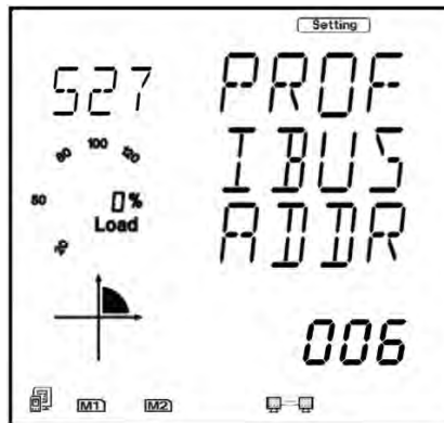
Figure 5-50 AXM-PROFI address setting on meter display
