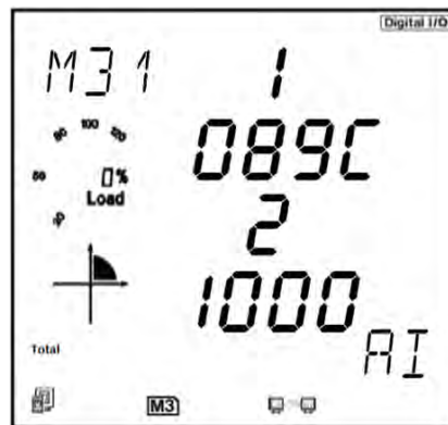
Figure 5-42 Analog Input reading from the meter display
