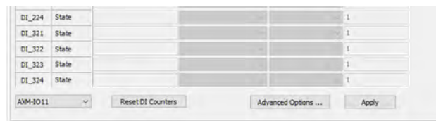
Figure 5-28 Reset DI Counter from Acuvue software
