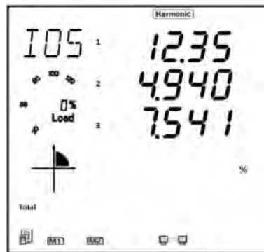
Figure 3-23 - Individual Harmonic Reading
