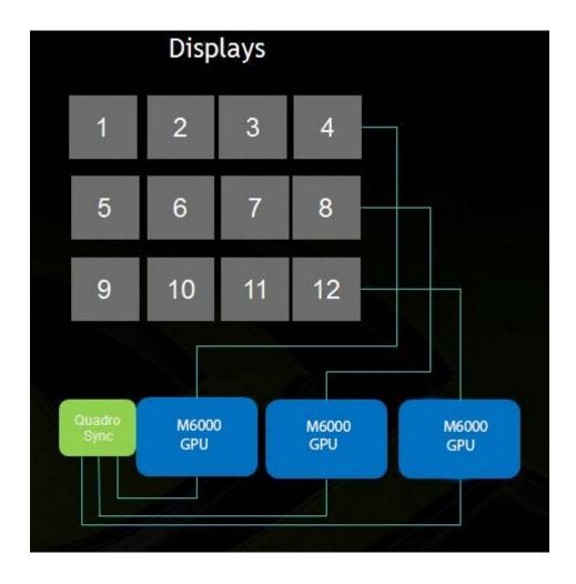
4) Sixteen (4 x 4) display configurations with four Quadro M6000s and Quadro Sync.
