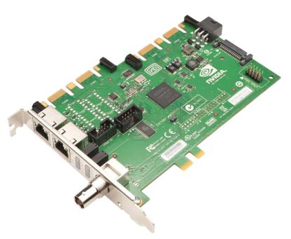
Refer to the NVIDIA Quadro Sync Quick Start Guide which covers the various connectors available and how to connect the Quadro Sync board to the Quadro M4000.
