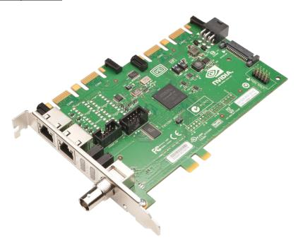
Refer to the NVIDIA Quadro Sync Quick Start Guide which covers the various connectors available and how to connect the Quadro Sync board to the Quadro K5200.
