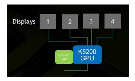
2) Eight (1 x 8 or 2 x 4) display configuration with two Quadro K5200s and Quadro Sync.
