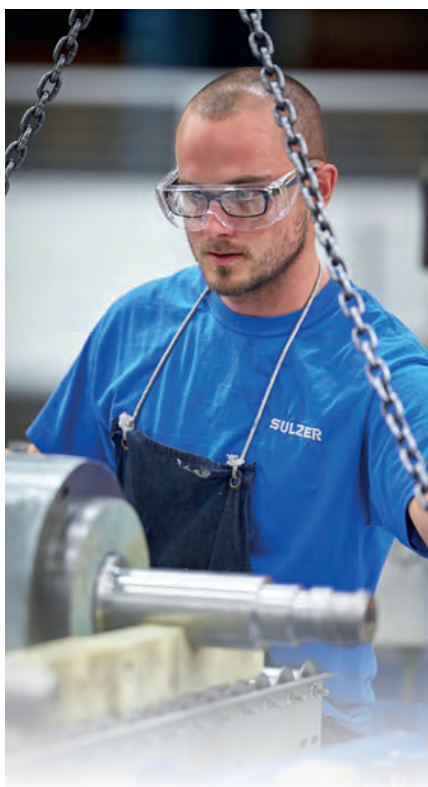
Sulzer's engineers refurbished the rotors and casing to OEM dimensions
