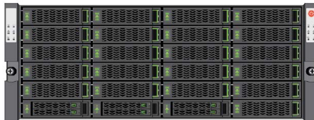
HPE Nimble Storage Adaptive Flash Array 3 (Base array, 4U; 21 bays hold carriers with Large Form Factor HDDs, 3 bays hold Dual Flash Carriers with Small Form Factor SSDs)
