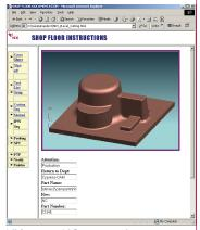
NX creates NC program documentation for use on the shop floor. The output can be configured to produce ASCII files, HTML (viewable from a web browser), and other formats.
