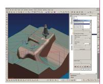
Fixed-axis core and cavity milling in NX Mach Series Machining Solutions creates toolpaths that remove material in planar layers perpendicular to the fixed tool axis.
