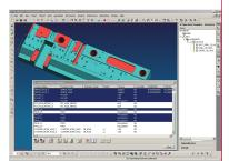
NX automates toolpath creation for machining holes, pockets, and faces with feature-based machining.
