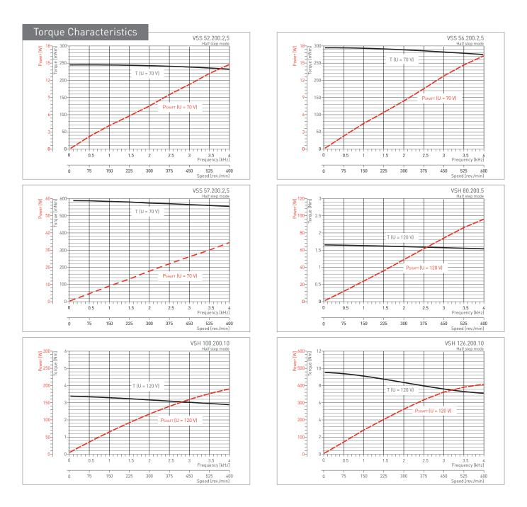
U= 70  $V_{DC}$  / 120  $V_{DC}$ : Operating voltage of the power stage (intermediate circuit voltage)
