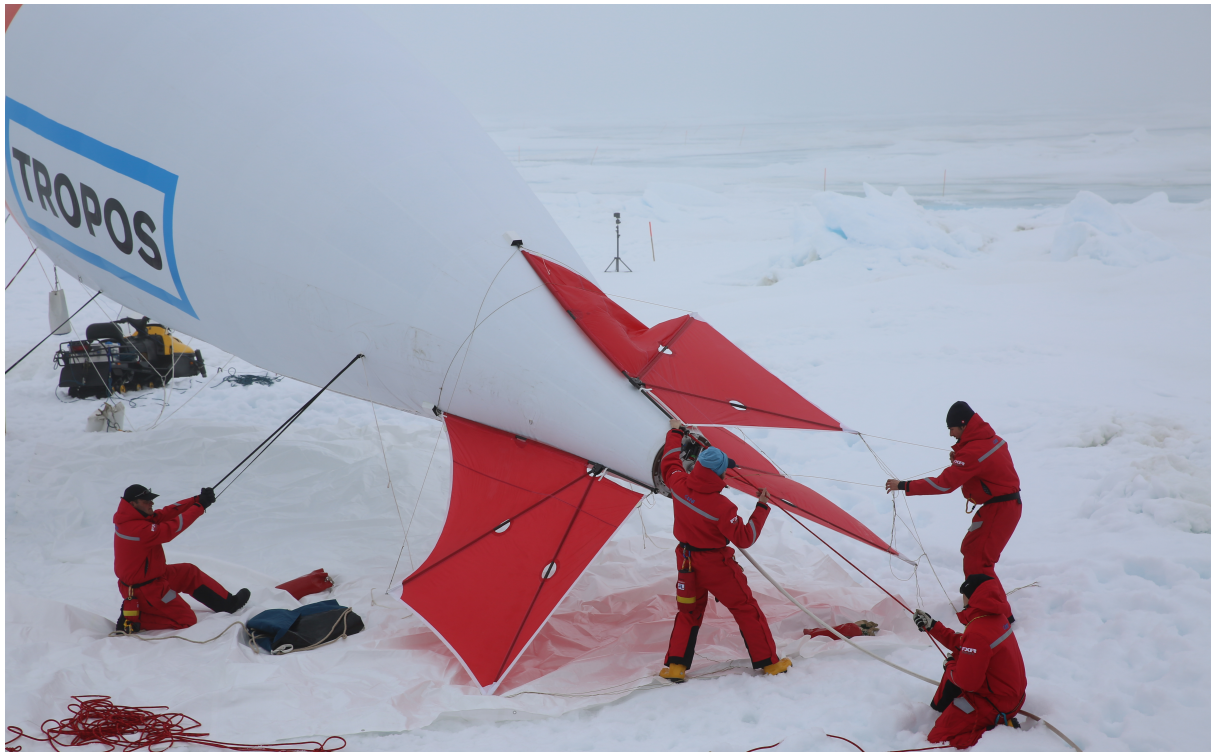
Figure 3: The complexity of the preparation and maintenance of BELUGA required the help from several volunteers during the whole deployment period. During these operations, the balloon was secured with ropes to a snowmobile and controlled by the volunteers. Credits AWI/Grosfeld.
