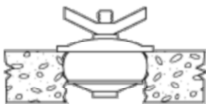
Plug openings in sewer access
