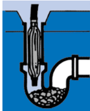
2. Insert Flusher into drain.
