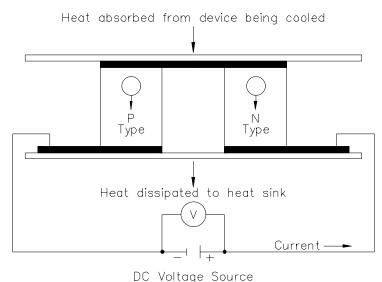
(bismuth telluride) between the plates. The elements of
