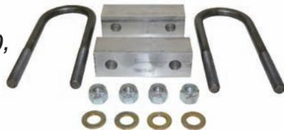
Obtain 2" of drop on your coil spring truck with our proven billet lowering block kit. This kit lowers the rear of your coil spring truck up to 2" without affecting your ride quality. These block kits allow the vehicle's shock angle to remain unchanged from the factory position. Works great with lowered coils to get that slammed look without sacrificing the handling characteristics. Available in 1", 1.5" and 2" drops. Please specify when ordering.
