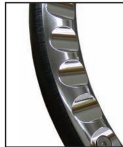
These wheels include finger grips on the backside for a comfortable drive.
