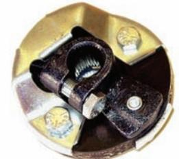
These rag joints are a must when converting to power steering. They eliminate road vibration and pump noise in your steering wheel. These rag joints are designed for use when running a stock "GM" steering column intermediate shaft. OEM Replacement. Economically priced. For all vehicles with 13/16" Diameter - 36 Spline.
