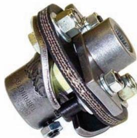
These rag joints are a must when converting to power steering. They eliminate road vibration and pump noise in your steering wheel. These rag joints may not work with certain power steering conversion kits.
