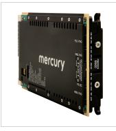
The 5560 is a high-performance, SOSA aligned 3U OpenVPX coprocessor board based on the Xilinx Versal HBM ACAP (Adaptive Compute Acceleration Platform). It serves as an ideal stand-alone processor or as a co-processor for distributed ACAP processing tasks.
