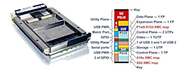
3. SOSA modules like Pentek's Model 71813 XMC module (left) are designed to work with OpenVPX-compatible VPX boards that provide standard connections to the backplane.
