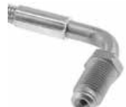
HE606-03P-090 90° 10x1.0mm male hose end with convex seat in unplated steel (mates to HE551-03P-000 at left)
