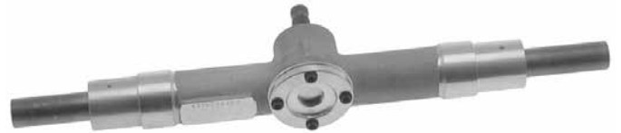
Stock Steering Rack, Part No. 1802 Dimensions of Stock Steering Rack: • 18" Rack Bar Length • 13" Housing Length • 10" Between Mounting Shoulders • 1.5" Housing Diameter at Mounting Bosses • \frac{1}{2} -20 UNF Female Threads on Rack Bar Ends
