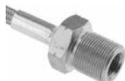
HE551-03P-000 10x1.0mm female hose end with concave seat for bubble flare and male threads for bulkhead mounting in plated steel
