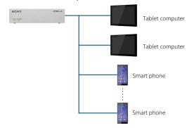
\*4 Up to 4 devices connection requires the optional software PCSA-MSA1, up to 10 devices the optional PCSA-MSA1 and PCSA-MPE1, and up to 16 devices the optional PCSA-MSA1, PCSA-MPE1, and PCSA-MPE2.
