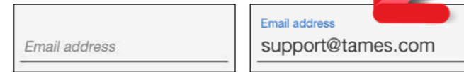
Example of an Edit control with "Hint text" that moves to the top when entering information
