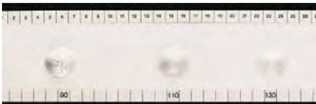
test panel is cured in the gradient-oven using the temperature profile of the production oven
