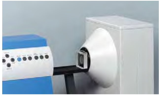
Liquids are best measured using cuvettes and the cuvette table.
