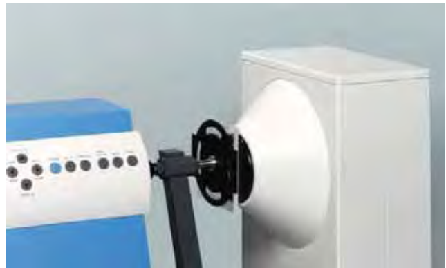
The measurement of haze is used to determine abrasion resistance of transparent materials. The Abrasion Holder facilitates positioning of the abraded area in the measurement beam.
