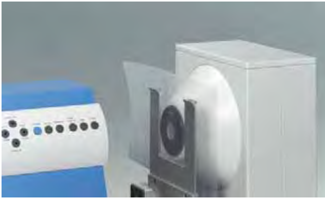
Exact positioning of films in the hazemeter with a holder guided in a precision track system.
