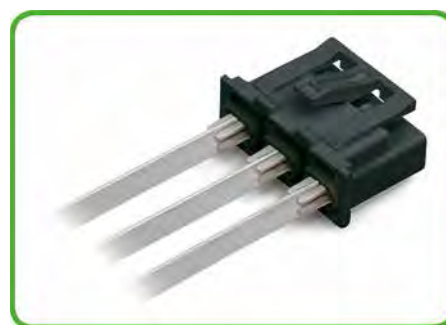
Device connectors can be cost-effectively installed in appropriate guide slots of a housing. Internal electrical connection is performed by contacting the 0.8 mm thick current bars. 2
