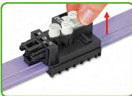
Lift contact element to unlock phase selector and select the new phase. NOTICE: Do not reuse in the same location of the flat cable.
