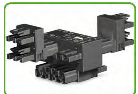
Additional h-distribution connectors double L1 and L3. This results in the following connection option: L1/L1/L2/L2/L3/L3 with jumper in position L2 NOTICE: h-distribution connectors can only be plugged on L1 and L3.
