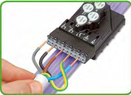
Connecting an installation cable to the supply module. Stripped, solid conductors are simply pushed into unit. Open clamp via screwdriver to insert stripped, fine-stranded conductors.
