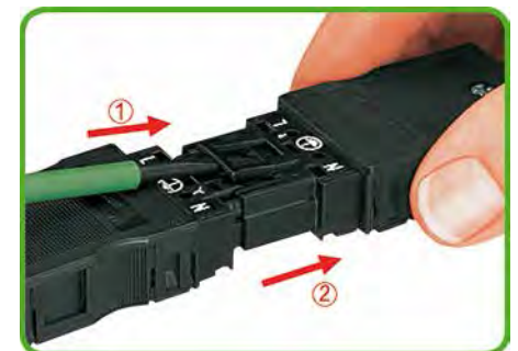
Locking lever, tool operated: 1.) Unlatch locking lever. 2.) Pull apart the connectors. (Example shows 3-pole connectors)
