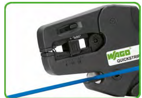
Cutting a conductor.
