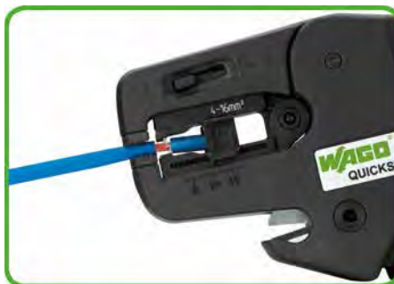
Stripping a conductor.
