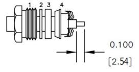
Click the following link (or enter part number in "SEARCH" on website) to obtain additional part information including price, inventory and certifications: BNC Male Connector Clamp/Solder Attachment for RG58, RG55, RG141, RG142, RG223, RG400, RG303, PE-C195, PE-P195, LMR-195 PE4023
