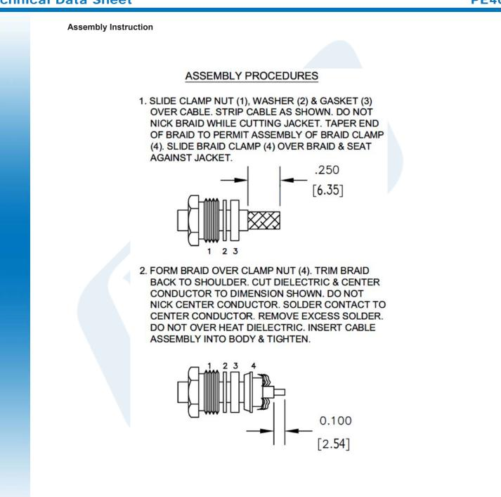
Click the following link (or enter part number in "SEARCH" on website) to obtain additional part information including price, inventory and certifications: BNC Male Connector Clamp/Solder Attachment for RG58, RG55, RG141, RG142, RG223, RG400, RG303, PE-C195, PE-P195, LMR-195 PE4023
