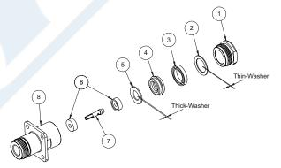
Click the following link (or enter part number in "SEARCH" on website) to obtain additional part information including price, inventory and certifications: N Female Connector Clamp/Solder (Captive Contact) Attachment 4 Hole Flange Mount for RG214, RG213, RG393, RG8, RG225, .718 inch Hole Spacing PE4060
