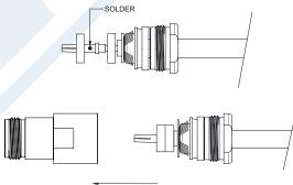
Click the following link (or enter part number in "SEARCH" on website) to obtain additional part information including price, inventory and certifications: N Female Connector Clamp/Solder (Captive Contact) Attachment for RG213, RG214, RG8, RG9, RG11, RG225, RG393, RG144, RG216, RG215 PE4059
